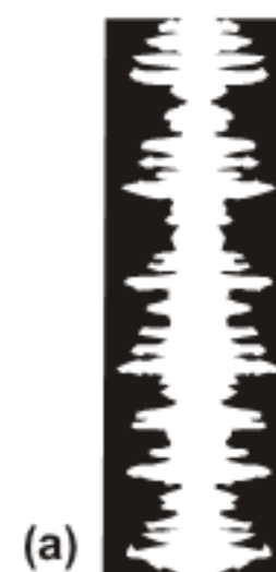
(a) Fig. Sound track on a film which varies the intensity of light reaching the photo cell.
